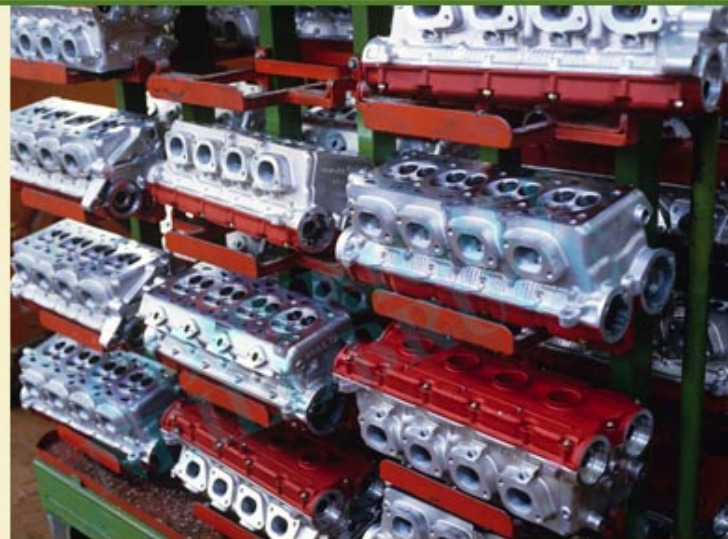
FF90019. V8 cylinder heads for 3.4 litre engines
