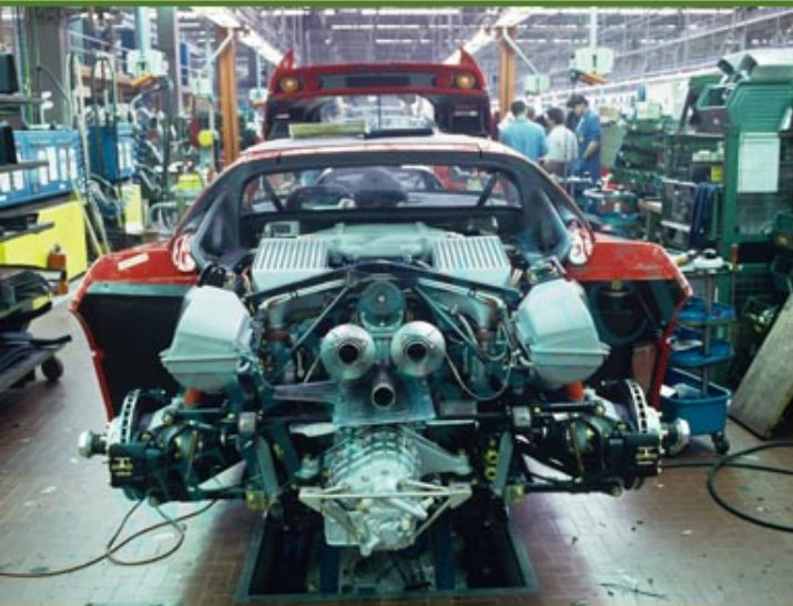
FF90100. Engine and drivetrain installed
