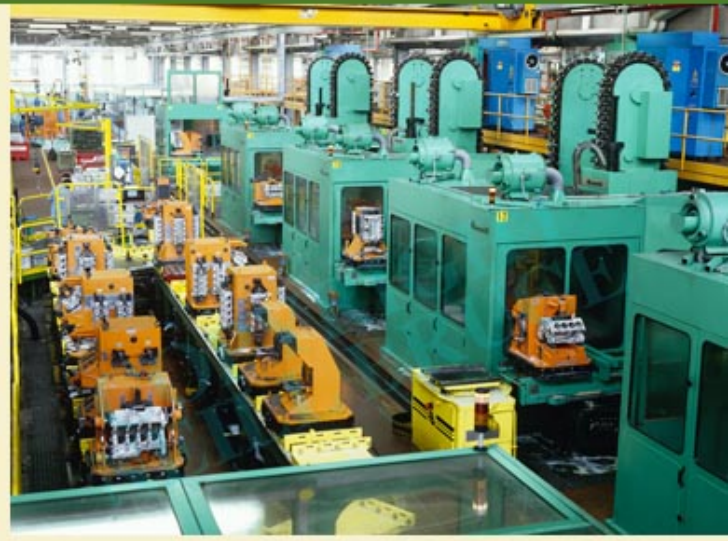
FF90006. V8 blocks and heads ready for machining
