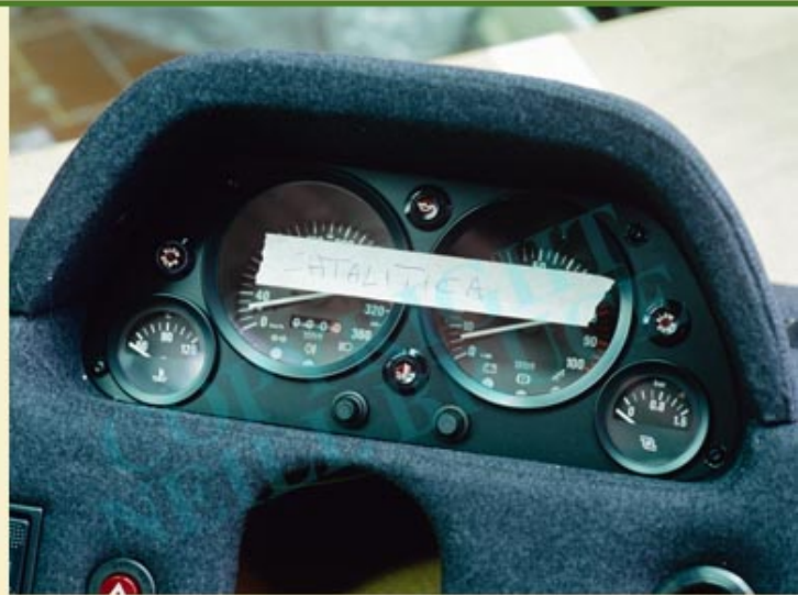
FF90129. Instruments for catalyst F40 Note "Slow Down" warning lights
