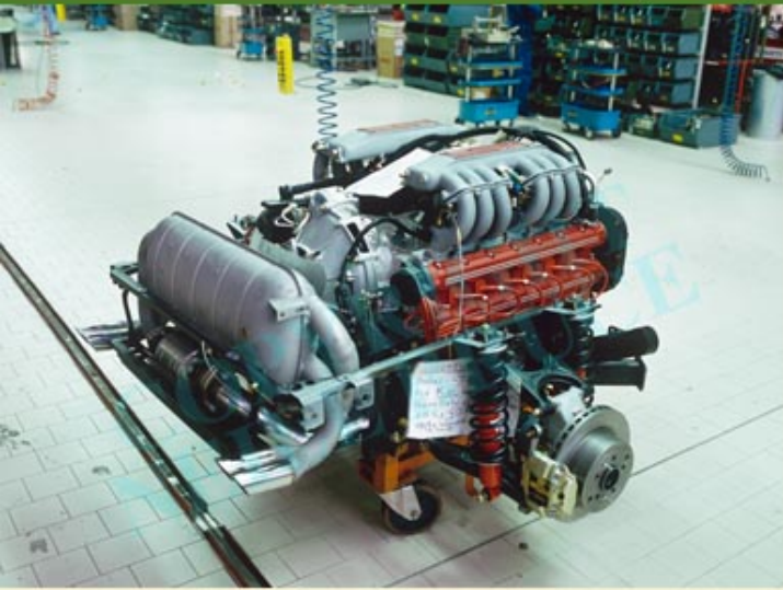
FF90142. Catalyst engine and drive system
