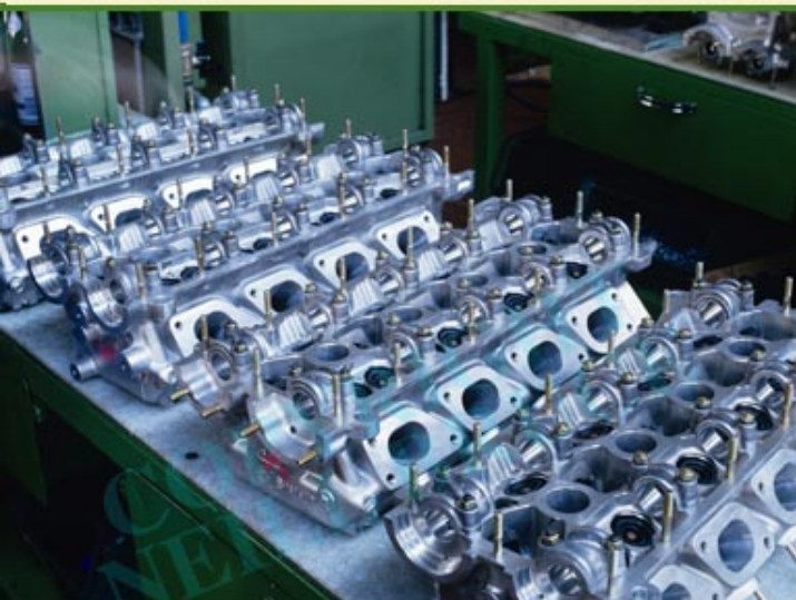
FF90017. V8 cylinder heads ready for camshafts
