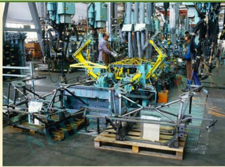
FF90056. 348 rear sub frames and jig
