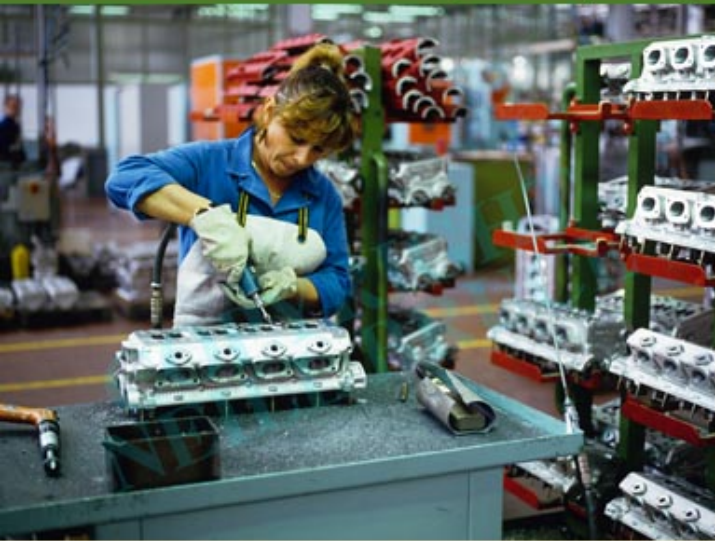
FF90014. De-burring a V8 cylinder head
