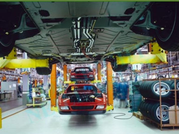
FF90086. Variable height assembly line
