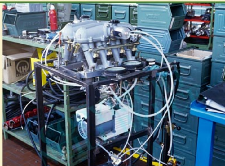
FF90051. Setting up fuel injection on a 3.4 litre engine
