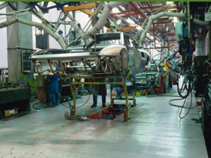
FF90067. Mondial tb robotic body welding
