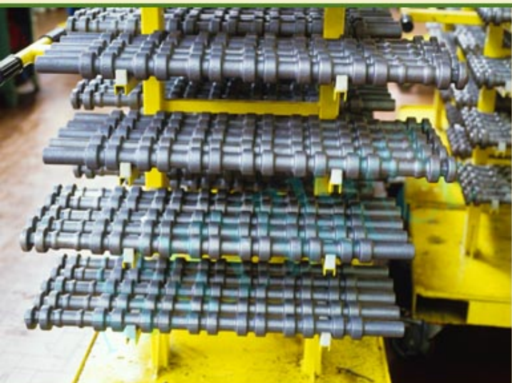
FF90020. Unmachined camshaft forgings
